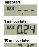
At Insulation Measurement Ranges, after a certain time passes since a measurement is started, the display automatically shows DAR/PI values.
